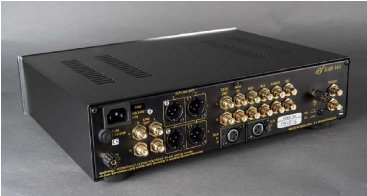
Double XLR outputs and a single pair of XLR inputs. Phono sockets are for an external phono stage.
